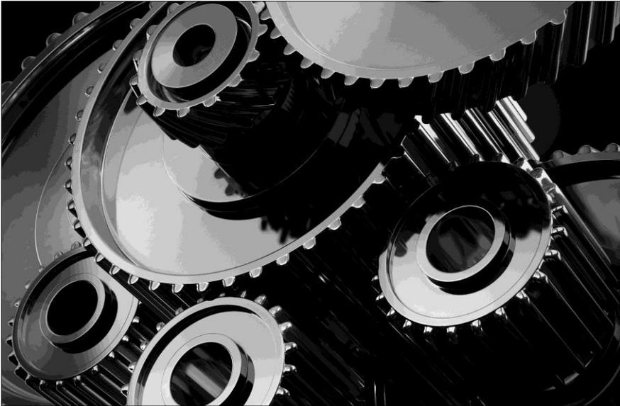
A gear or cogwheel is a rotating machine part having cut teeth, or cogs, which mesh with another toothed part to transmit torque, in most cases with teeth on the one gear being of identical shape and often also with that shape on the other gear. Two or more gears working in a sequence (train) are called a gear train or, in many cases, a transmission; such gear arrangements can produce a mechanical advantage through a gear ratio and thus may be considered a simple machine.
